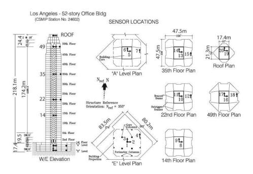
Figure 5. Schematic of vertical section and plan views as well as accelerometer deployment locations (from http://www.stronmotioncenter.org/, last accessed November 29, 2018)
