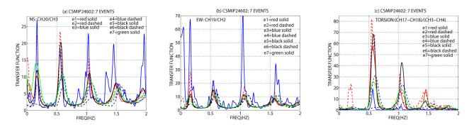
Figure 9. Transfer functions computed from amplitude spectra of accelerations at the roof and basement for 0-2 Hz bandwidth respectively in (a) and (b) NS direction (CH20/CH3), (c) and (d) EW direction (CH19/CH2, respectively and (c)torsion ((CH17-Ch18)/(CH3-CH4)).
