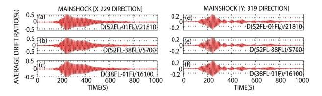
Figure 4. Average drift ratios computed from displacements between 52nd, 38th and 1st floors. In each frame, the numbers in denominators are distances (in cm) between the designated floors.
