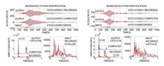
Figure 3. System identification applied to mainshock records. First-floor accelerations are used asinput and 52nd-floor accelerations as output. The computed 52nd-floor accelerations match well those that were recorded.
