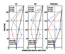
Figure 10. Three for each of NS, EW and torsional modes using Landers earthquake accelerations. Identified frequencies and critical damping percentages (abbreviated as dmp) are also shown.
