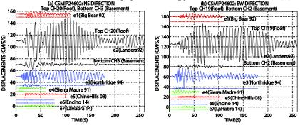
Figure 8. Equiscaled displacements at basement and roof of the building for seven events: (a) NS, (b) EW direction.
