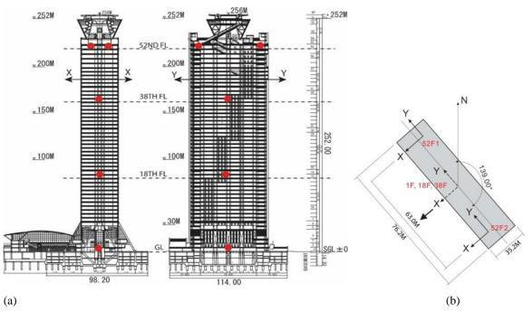
Figure 1. (a) Vertical sections of the building showing major dimensions and locations of tri-axial accelerometers on the 52n, 38th, 18th and ground level (1st Floor). (b) X and Y denote principal axes of the building and orientations of the accelerometers (from Çelebi et al, 2012[4]).
