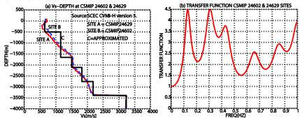
Figure 6. (a) Vs-depth profile [from SCEC CVM-H version 5.3] for downtown Los Angeles [Site A (red line) and Site B (dashed black line)] represent sites of tall buildings with CSMIP station numbers 24602. The profile C (step-line) represents approximated profile for both building sites. Alternate variations of approximations of step-profile should not alter the results significantly. (b) Transfer function is computed using approximated step profile C.
