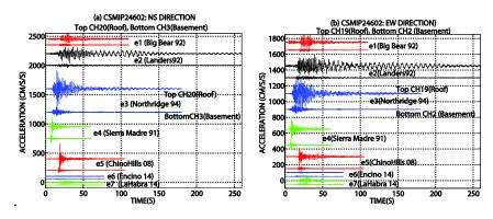
Figure 7. Equiscaled accelerations at basement and roof of the building for seven events: (a) NS, (b) EW direction. (a) CSMIP24602: NS DIRECTION (b) CSMIP24602: EW DIRECTION
